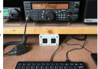
This interface allows the ham operator to set up the call and virtually 'pass the mic' to a Zoom-connected Scout to exchange a greetings message. The Scout can be anywhere. The interface will allow a large number of Scouts to qualify for part of their Communicator Activity Badge, logging 25 stations.
